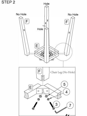
Attach (2) Chair Legs with No Hole (Part F) to the Apron with Swivel Plate (Part E), using (4) M6x45mm Hex Screws(Part 3), (4) Lock Washers, (Part 4) and (4) Flat Washers (Part 5). Loosely tighten with Allen Wrench (Part 7).
