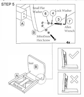
Attach the Backrest (Part A) to the Seat (Part B) using (4) M6x45mm Hex Screws (Part 3), (4) Lock Washers (Part 4) and (4) small Flat Washers (Part 6). Tighten loosely with Allen Wrench (Part 7).
