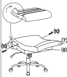
Open the Velcro on both sides of seat first, then place the Back Cushion(7) on the Seat Cushion (6), and use 2 bolts (10) to attach to the lower screw holes on Seat Cushion (6) (see diagram).
