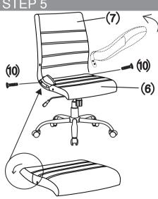
Push the Back Cushion (7) up to a vertical position and attached the Seat Cushion(6) to by using 2 bolts(10), then to cover the Velcro back.
